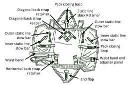
The pack tray holds the parachute, packed in the deployment bag, to the parachute harness. It is constructed of nylon duck. The waistband is located near the bottom of the pack tray.
