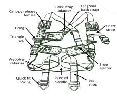
The parachute is attached to the harness assembly, which secures the parachute to the paratrooper before the jump and during the descent. The harness assembly is equipped followings:
