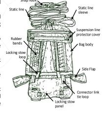
The static line has single action snap hook at the end and the other end is tied (or stitched) to deployment bag.
